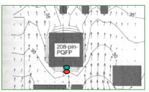
Figure 7b. Dual Sensor HWA Used to Measure  $V_{_{\alpha}}$  and  $T_{_{\alpha}}$  for Calculating Junction Temperature
